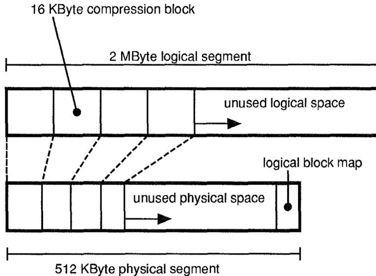
Figure 2: Logical and physical views of a segment.
